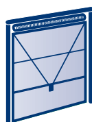
Canopy gear (C) for single doors
