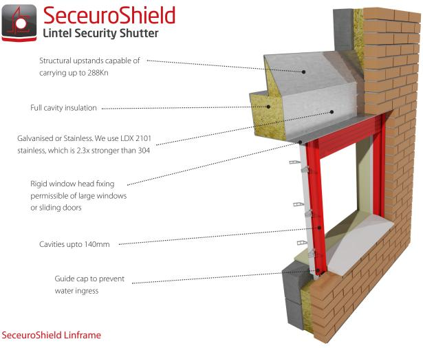
The Linframe is an FCS (full closer system). This provides a complete insulated closer for an aperture which closes the bottom of the shutter's guides, allowing a weather seal finish. Rigid UPVC elbows set an opening size to the exact dimensions required.
