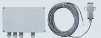
2-channel relay receiver HER 2 With 2 volt-free relay outputs, frequency: 868 MHz, IP 65, operating voltage: 24 V DC / 230- 240 V AC, separate antenna for exterior use (IP 65), in a tamper-proof aluminium housing with 7 m connecting lead, 3-wire, decoder unit for interior
