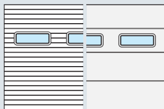
With compound window type A Door section heights: 500, 625, 750 mm
